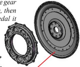
Ford Model A Flat Rattler for “preselector” gearbox. This is a bit different as this user had a preselector gearbox, but shows the Rattler as a bolted onto the flywheel.
