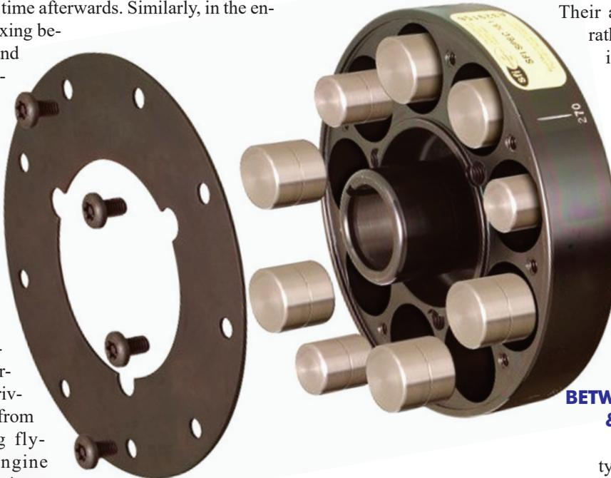
*Solid rollers are made in a variety of diameters and chosen to tune the balancer to the engine's requirements. This assembly is attached to the crankshaft nose or machined into a flywheel. It can incorporate a pulley and timing marks.*
